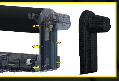
change sheet metal part for new one and mount holder - be carefully about holder direction
